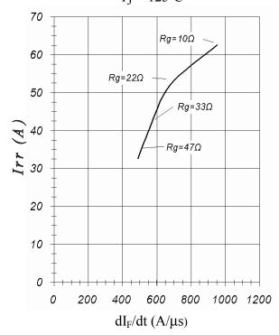
Fig. 18 – Typical Diode  $I_{RR}$  vs. Rg  $I_F = 30A$ ;  $T_i = 125$ °C
