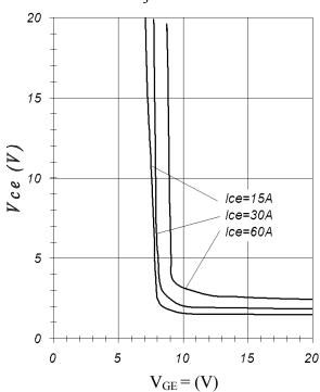
Fig.  $11 - \text{Typical V}_{\text{CE}} \text{ vs. V}_{\text{GE}}$  $T_i = 125^{\circ}\text{C}$
