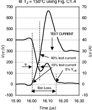
Fig. WF4- Typ. S.C Waveform
