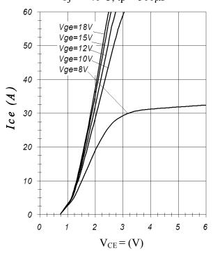
Fig. 7 – Typical IGBT Output Characteristics  $T_i = 125$ °C;  $tp = 500 \mu s$
