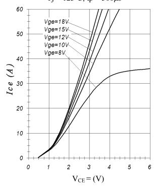
Fig. 6 – Typical IGBT Output haracteristics  $T_i = 25$ °C;  $tp = 500 \mu s$
