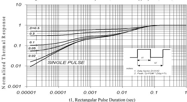
Fig. 25 – Normalized Transient Impedance, Junction-to-copper plate (IGBTs)
