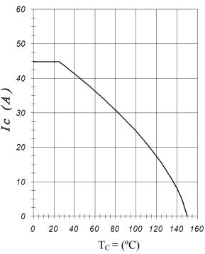
Fig. 3 – Forward SOA  $T_C = 25^{\circ}C$ ;  $T_j \le 150^{\circ}C$
