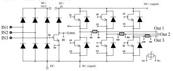
Three phase bridge brake inverter with current sensing resistors on all output phases and thermistor
