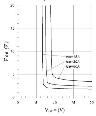
$\begin{aligned} \text{Fig. } 10 - \text{Typical } V_{\text{CE}} \text{ vs. } V_{\text{GE}} \\ \text{Tj} &= 25 \text{°C} \end{aligned}$
