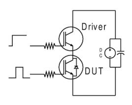
Fig. CT.4 - Switching Loss Circuit
