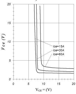
Fig. 12 – Typical Transfer Characteristics  $V_{CE} = 20V$ ; tp =  $20\mu s$
